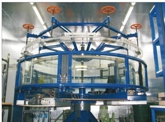
**Figure 2.2** Annular flume at the Institute for Hydraulic Engineering and Water Resources Management, Aachen, Germany.
